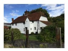
large stack to centre. Pentice roof, whitewashed brick extension to rear with first floor bracing exposed on rear of main house.
